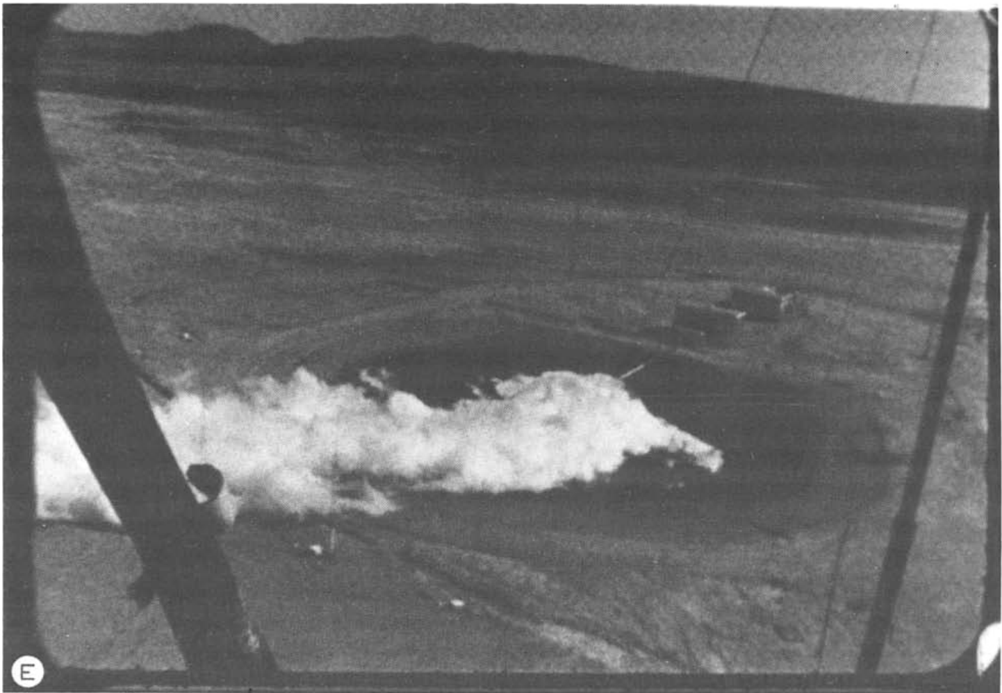
Fig. 7. Photographs of Burro 8 vapor cloud at (a) t = 2 s, (b) t = 30 s, (c) t = 80 s, (d) t = 160 s, (e) of Burro 6 vapor cloud after quasi-steady state had been reached. Spill rates were similar in both tests ( 16 \text{ m}^3/\text{min} in Burro 8 and 13 \text{ m}^3/\text{min} in Burro 6). The main difference between the two tests was the more stable atmospheric conditions and lower wind speed ( 1.8 \text{ m/s} vs. 9.1 \text{ m/s} ) in Burro 8 test.
